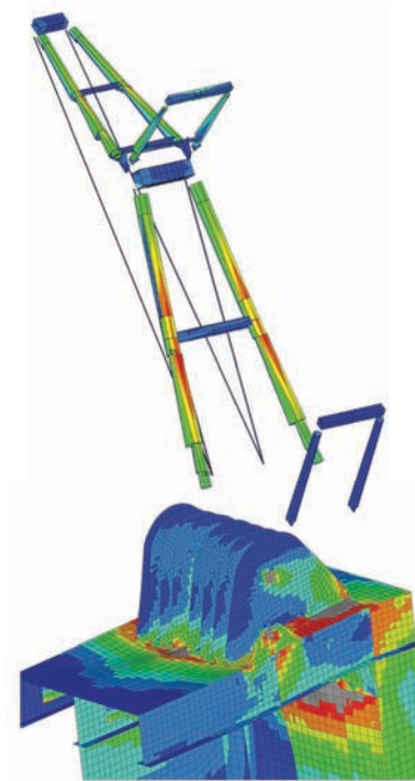
Finite element analysis calculated stress distribution in the overall Matador 3 lifting structure (top) as well as individual critical components such as the sheave support plates (bottom)
