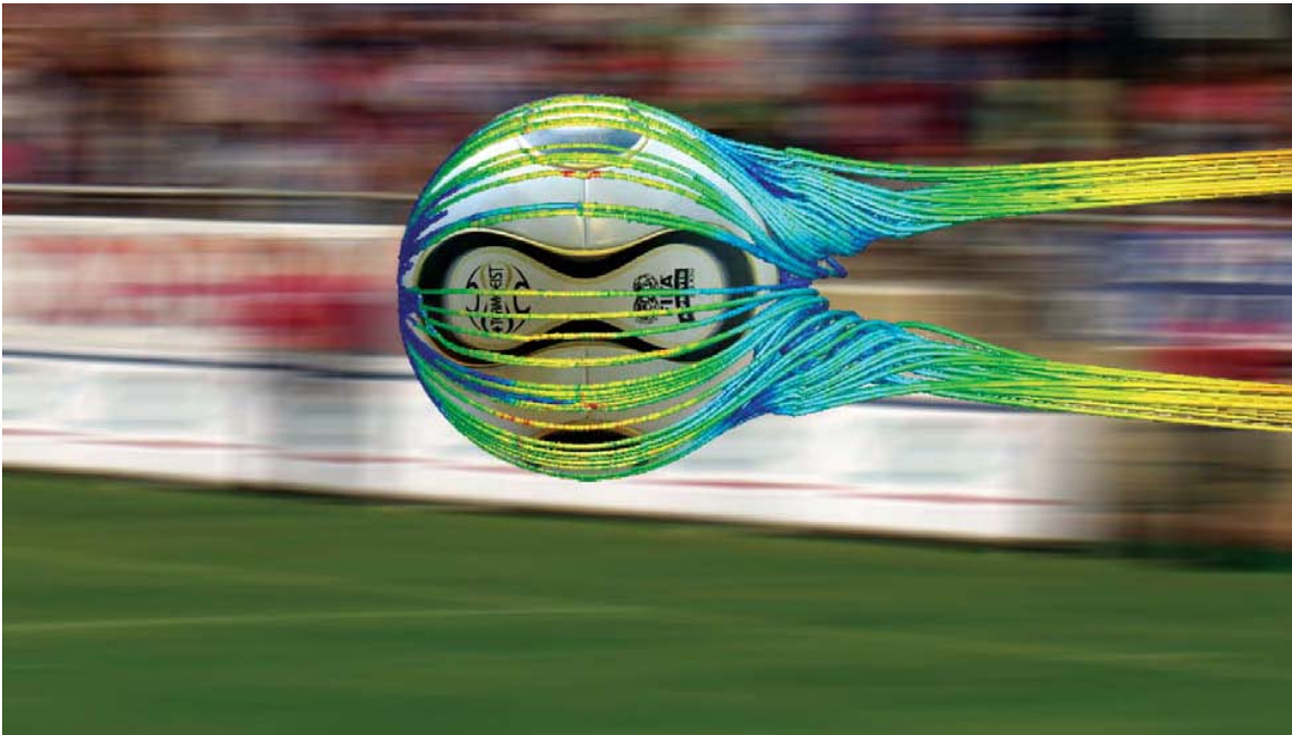
Pathlines colored by velocity show the detailed flow field surrounding a soccer ball in flight
