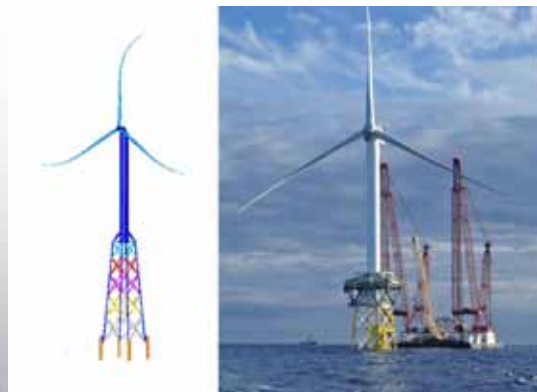
Nonlinear dynamic analysis of offshore wind turbine structure Courtesy REpower Systems AG.
