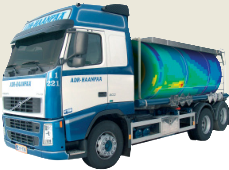
A liquid-hauling tank and associated structures of the truck were analyzed. The truck's tank was made of filament-wound composites and sandwich structures.
