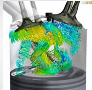
Vortex structures in a four-stroke engine just after injection of fuel and intake valve opening Courtesy of BMW Group.
