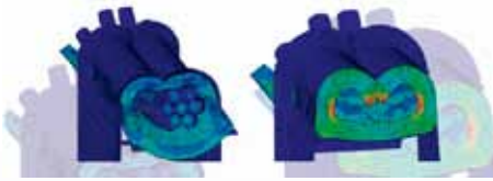
Crimping of wires
