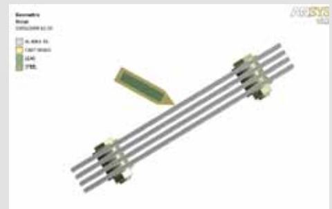
Reinforced concrete beam with loading resulting in failure
