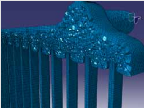
The hybrid mesh in a car engine radiator
