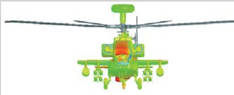
Contours of pressure on a helicopter in hovering flight mode
