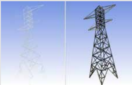
Simplified beam model representing an electrical tower
